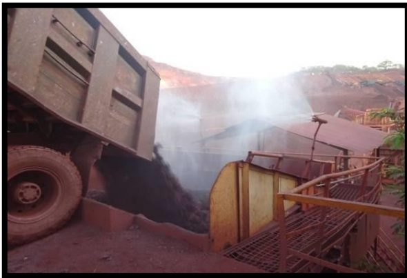
A photo showing dry fog implementations at various plants.
