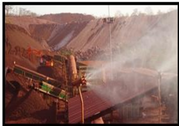
A photo showing dry fog implementations at various plants.
