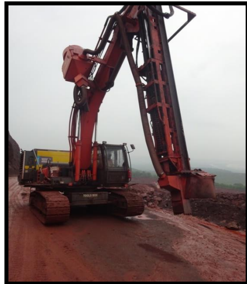
Photo Showing Excavated Mounted Drilling Machine equipped with dust extractor & wet drilling mechanism
