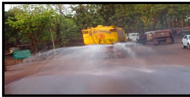
Photo showing 16 Kl water tanker engaged in Village road dust suppression
